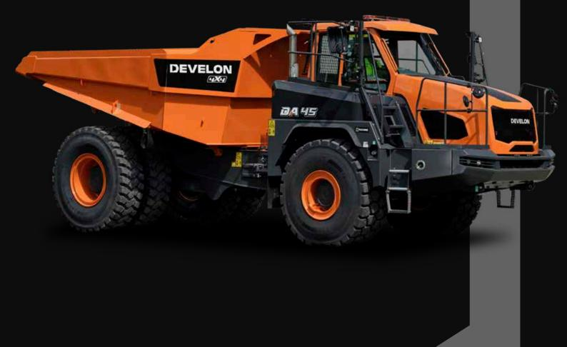
Maximum power500 hpOperating weight71.5 tBody capacity25.7 m<sup>3</sup>
