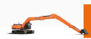
**Super-long reach and two-piece boom:** one long-reach machine — with a reach of 17.5 m — is ideally suited for special applications. A two-piece boom machine configuration is also available for more versatility.
