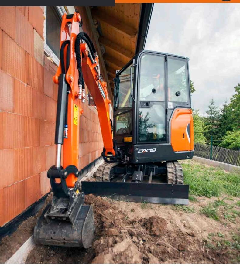
Maximum power: 13.3 hp Operating weight: 1.9 t Max. bucket capacity: 65 l
