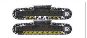
**Track guards:** to provide better protection, track alignment, and performance of machine while travelling. 3 guards per track as standard or DX49oLC-7 & DX53oLC-7 (full-length track guard optional) and, for DX42oLC-7, 2 guards per track as standard (double and full-length track guards available as options). These various track guard options provide you with optimal solutions for your extreme applications.
