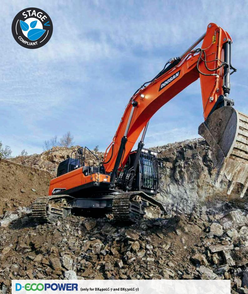
Real breakthrough technology that sets new standards in the industry: The exclusive ECO Power system improves productivity and saves fuel. A pressure-controlled pump, closed-center main control valve, and 9 sensors electronically detect and control the precise amount of hydraulic oil required to perform a task. The exact amount of oil required is metered instead of continuously forcing a fixed amount of oil through
