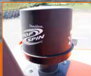
Centrifugal pre-cleaner Top Spin™ Donaldson® series
