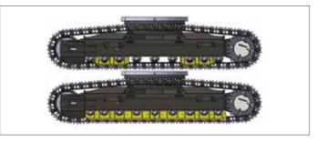
**Track guards:** to provide better protection, track alignment, and performance of machine while travelling. 3 guards per track as standard for DX490LC-7 & DX530LC-7 (full-length track guard optional). These various track guard options provide you with optimal solutions for your extreme applications.
