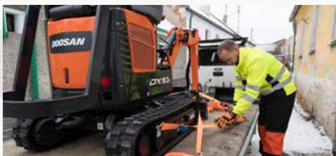
**Transportability:** The DX10Z fits easily on a conventional trailer. Easier transportability with new integrated upper structure tie-down points.
