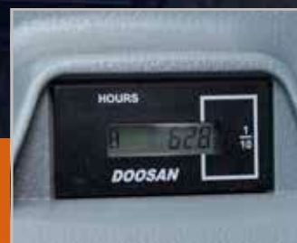
Hour meter (readable from ground level)
